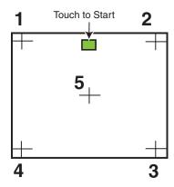
Figure 17. Sequence of Cross Positions for Setting the Touch Accuracy of a Screen
